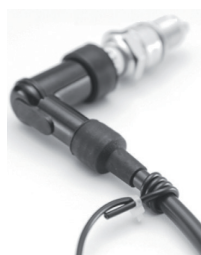
2/4 stroke install: Wrap pickup wire around spark plug lead.
