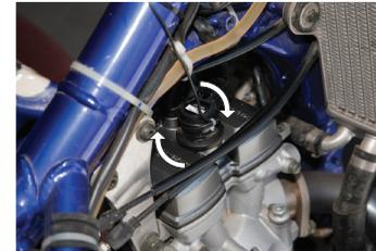
4 stroke installation, wrap pickup wire around head of coil...it's that easy!
